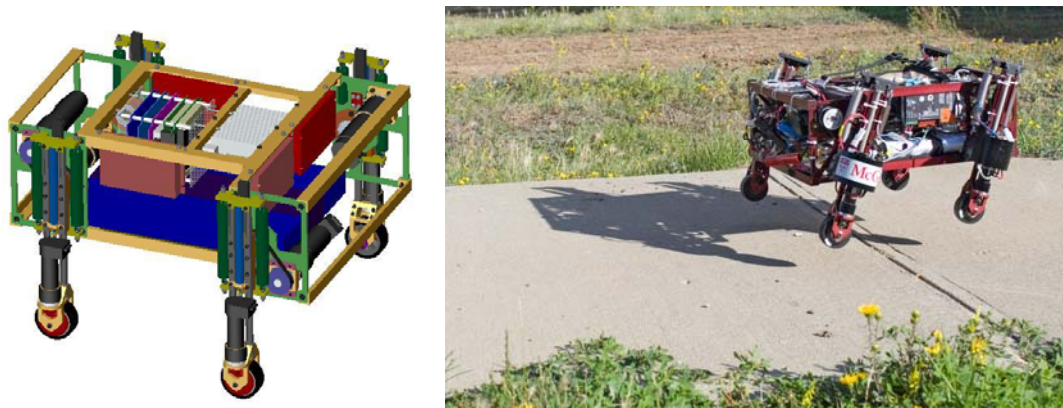
Figure 4: (left) CAD design of dynamic reactive platform concept. (right) First implementation of a dynamically stable bounding gait on a hybrid wheeled-leg robot.
